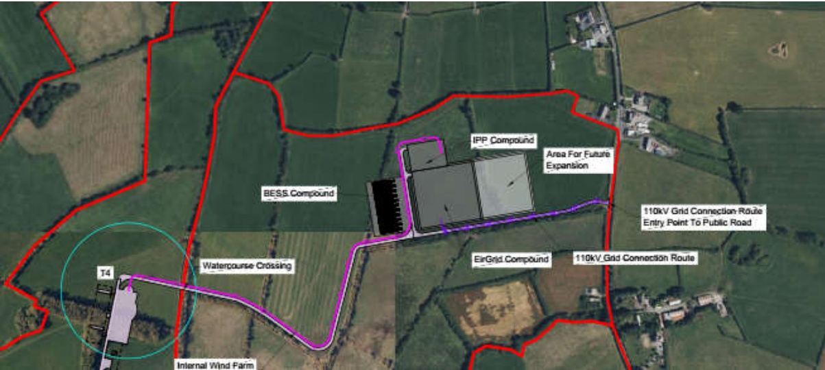
Figure 4-21: Second Proposed Substation and BESS Location
