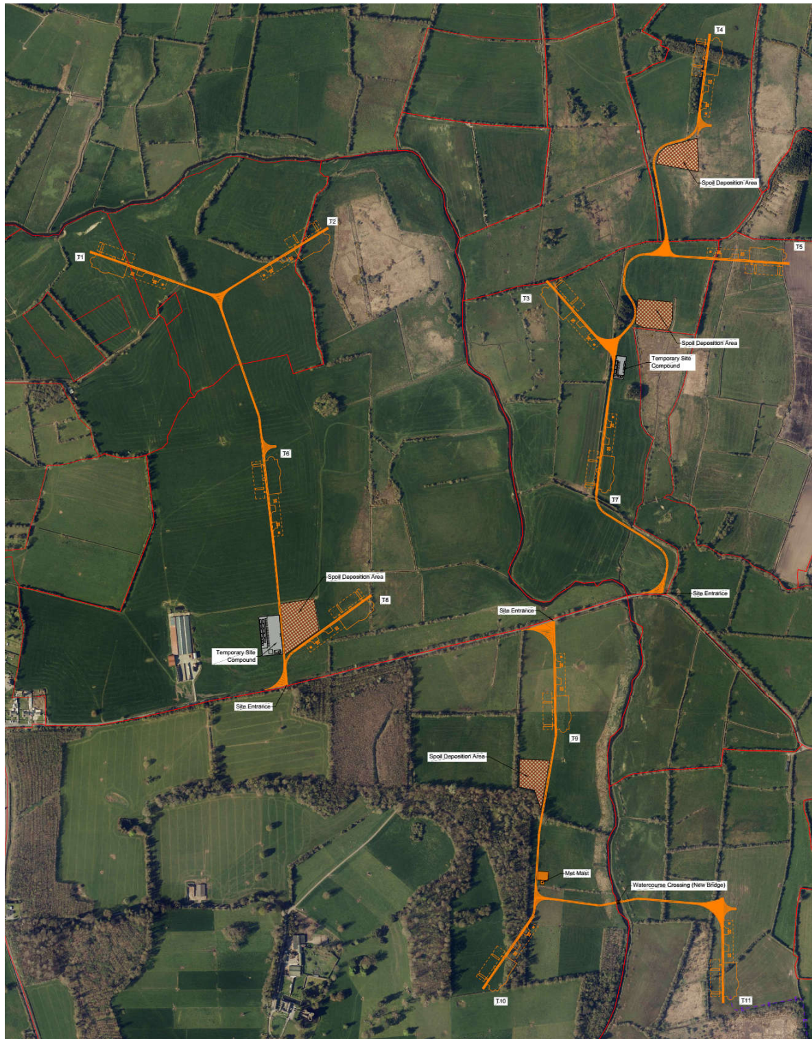
Figure 4-17: Iteration 2 – 11no. Turbine layout with 180m Tip Height Turbines with access to T11 over the River Suir
