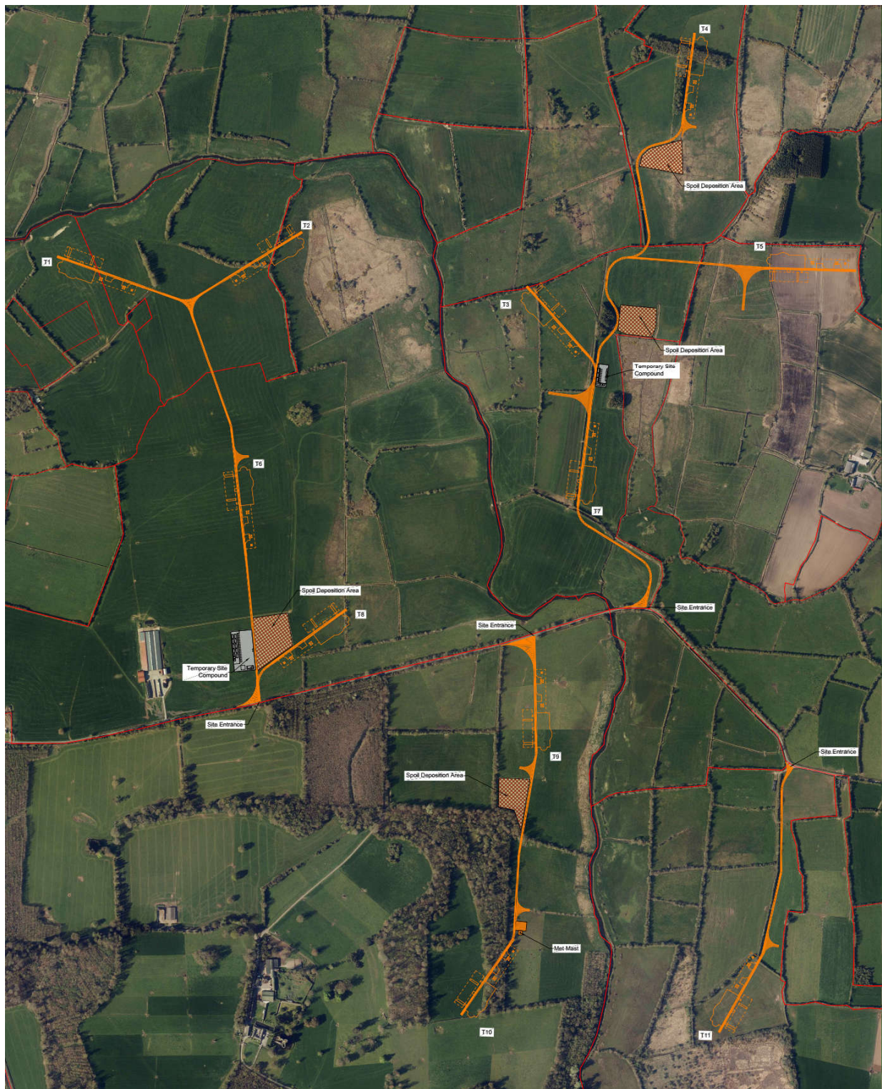
Figure 4-16: Iteration 1 Layout – more streamlined 11no. 180m Tip Height Turbine Layout
